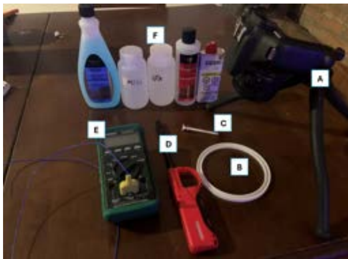
Fig. 2: Image of the setup used to make measurements. On the right is a DSLR camera (A) capable of shooting 1ms exposure. Next to the left is the 3D-printed channel (B). Above it is a syringe used to take out 0.1mL of fuel at a time (C). To the left of that is a lighter used to ignite the fuel (D). Finally, on the left is a temperature meter and thermocouple that were used to measure the temperature of the fuel after burning nearly to completion (E). On top (F), the fuels used are the methyl acetate/water mixture, methanol, isopropyl alcohol, acetone and zippo lighter fluid. Not shown, the phone camera used to record slow motion video.
